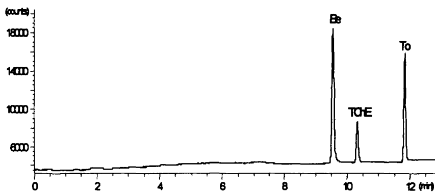
FIGURE 5 b) FID chromatogram of spiked gas sample injected after 60 min of the permeation from the water sample performed on the capillary column CP Sil 5 CB (25 m × 0.32 mm i.d. × 5 μm film thickness) under TPC: initial temperature 27°C – 1 min, temp. grad. 13°C/min, final temperature 180°C – 5 min, carrier gas helium (24 cm/s), temperature of FID 280°C. Peaks: Be – benzene, TChEt- trichloroethylene, To – toluene
